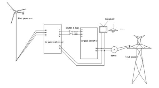
Notes : ① whether the generator can be incorporated into the power grid rests on local laws and regulations .
